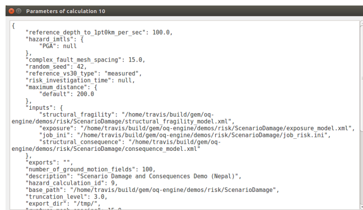
Fig. 14.3: Example showing parameters of a OQ-Engine calculation
