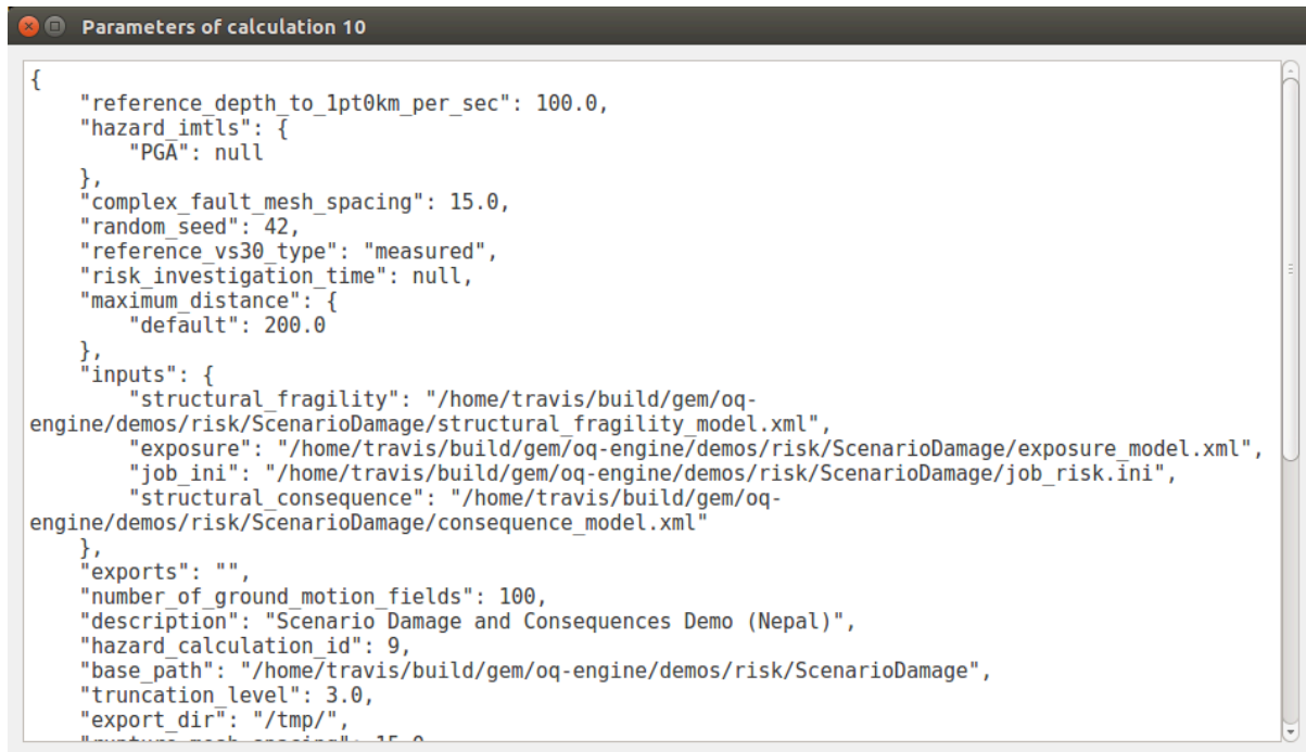
Fig. 15.3: Example showing parameters of a OQ-Engine calculation
